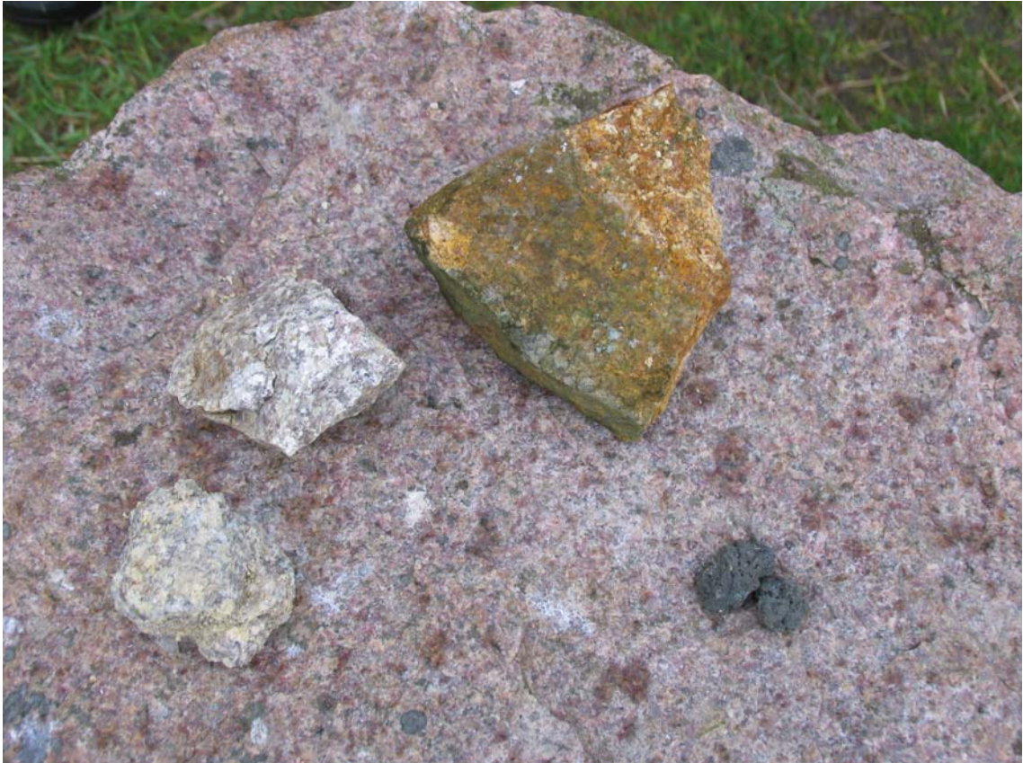
Figure 39. Fine-grained Hammer Granite. The four smaller fragments represent different levels in the weathering process of the granite: One fragment with yellow brown weathering of iron oxides, two grey and white fragments in different degree of kaolin weathering and one black fragments of manganese oxide formed in a fracture.
